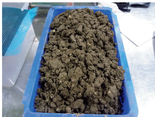
(3) Fiber-Cement-Stabilized Mud completion
